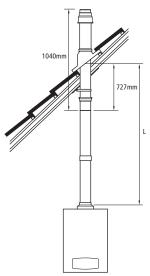
$\mathbf{L}$  = Flue length, measured from the top of the boiler to the underside of the roof flashing.
