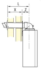
L = Flue length, measured from outside wall face to centre line of flue outlet. If L is less than 589mm then only the horizontal flue is required.
