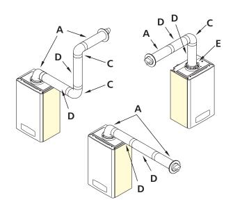
100mm diameter flue components as the horizontal flue options. The vertical flue adaptor **E** is required for vertical flue connections to the boiler.
